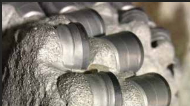
Figure 6. Resulting carbide substrate condition after drilling 8 legs of an oilsands well with a 7 7/8 SH513D PDC drill bit.
