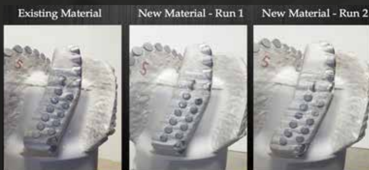
Figure 4. Comparative gage pad wear for three runs of the same bit in the same application with different coating technologies.
