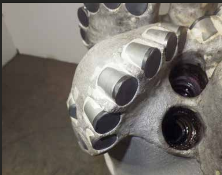
Figure 1. Dull condition of 6 ¼ in. SH513E PDC drill bit after drilling 1754 m in a challenging horizontal interval.
