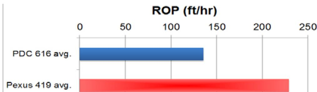
Figure 6. Average ROP comparison of 11 close offset 12 ¼ in. diameter intervals.
