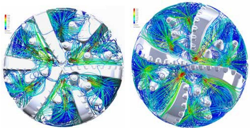
Figure 3. CFD comparison between Generation 2 (left) and 3 (right) Pexus hybrid designs.
