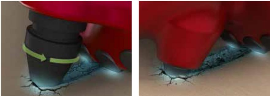
**Figure 1.** Pexus hybrid gouging/shearing cutting mechanism using either rotating (left) or fixed (right) inserts.
