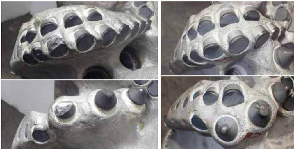
Figure 5. Dull condition of a 8 ¾ in. Pexus hybrid bit after completing a challenging reaming and vertical section (left). Dull condition of a 6 ¼ in. Pexus hybrid directional bit after completing a challenging build section (right).
