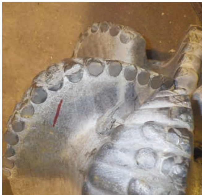
Figure 4. Gravel damage on a conventional large diameter PDC bit.
