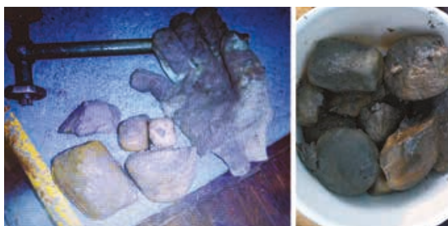
Figure 6. Rock samples from the first wells drilled by the new hybrid gouging/PDC bits.
